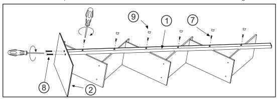
2)Please screw first the elliptic profile on the shelves and then screw the baseplate to this profile as shown in the figure 2.
